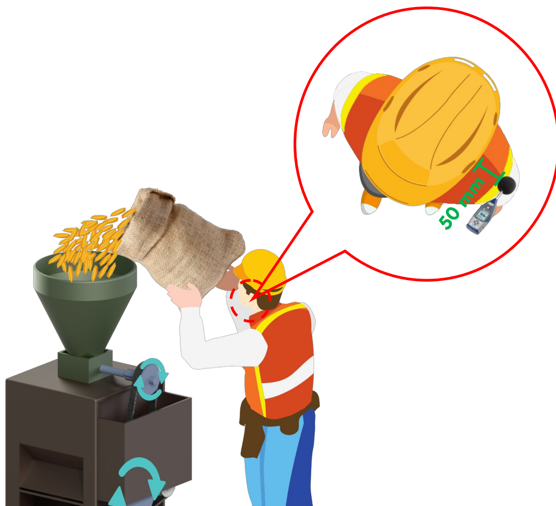
Figure 7. Measuring of Noise Level at Operator's ear
