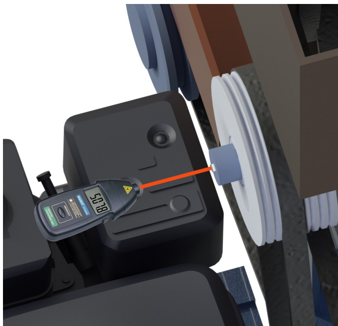
Figure 10. Measuring the speed of the rotating shafts
