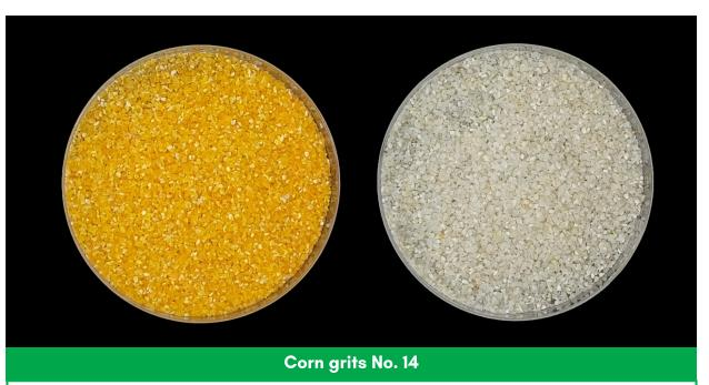
corn grits with particle size from 1.20~mm to 1.41~mm which passed through US Sieve No. 14 but are retained in US Sieve No. 16
