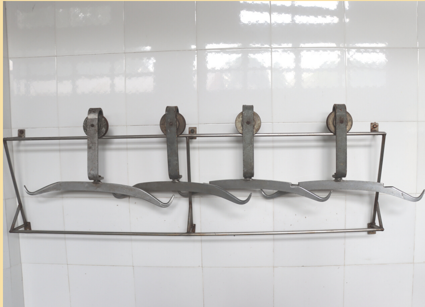
Image 50. Gambrel for pork carcass (Source: BAI-APDC, n.d)
