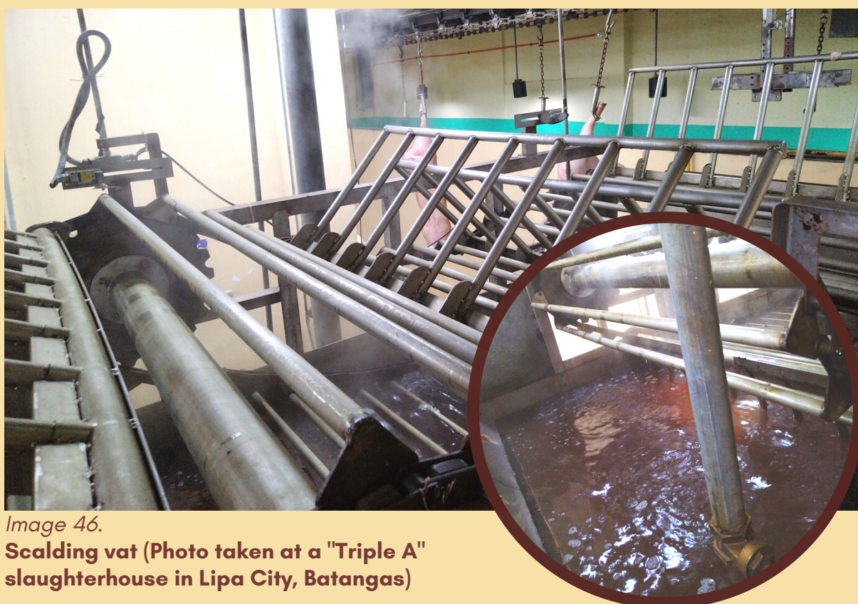
Image 45. Scalding vat/scalder (Source: NMIS, n.d)
