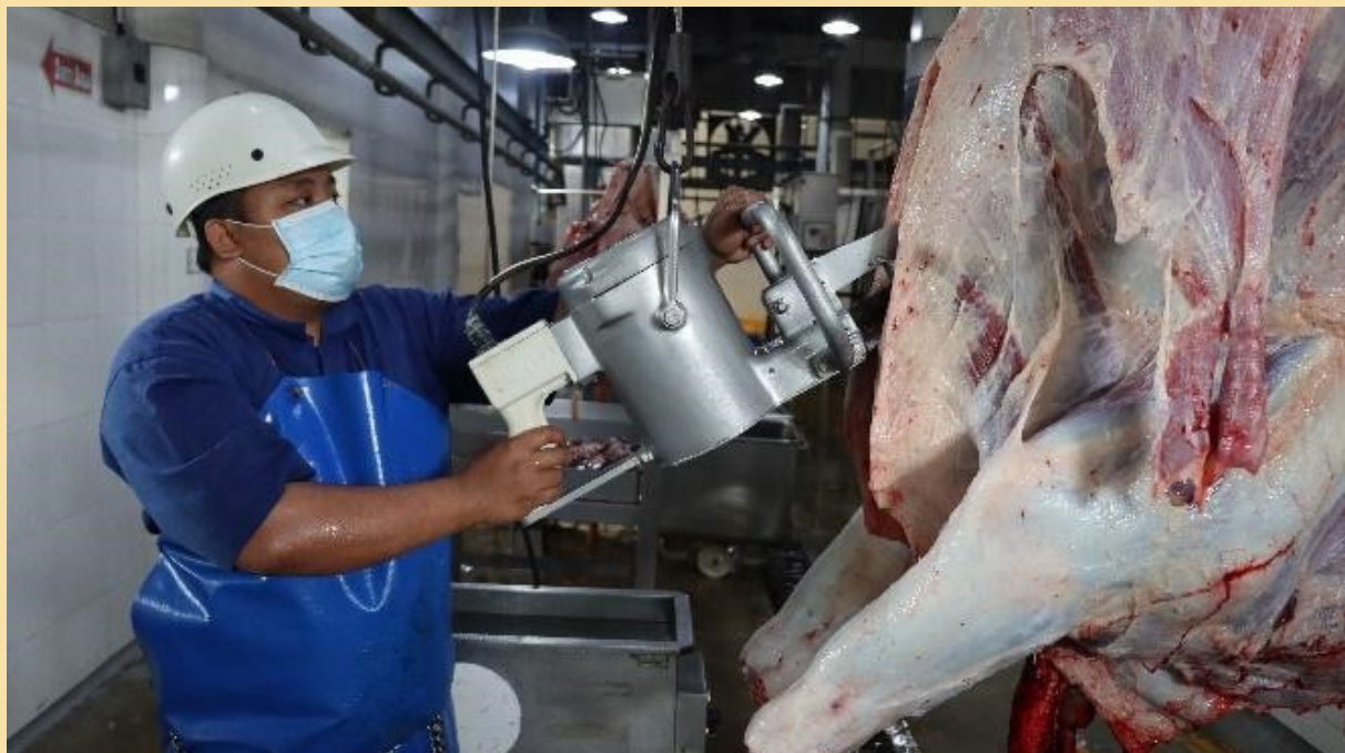
Image 44. Functional and easy to clean brisket saw for cattle (Source: BAI-APDC. n.d)
