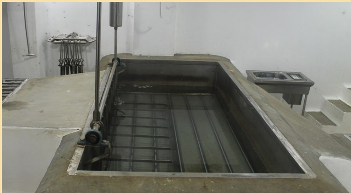
Image 45. Scalding vat/scalder (Source: NMIS, n.d)
