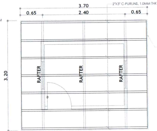
ROOF FRAMING PLAN SCALE 1:40
