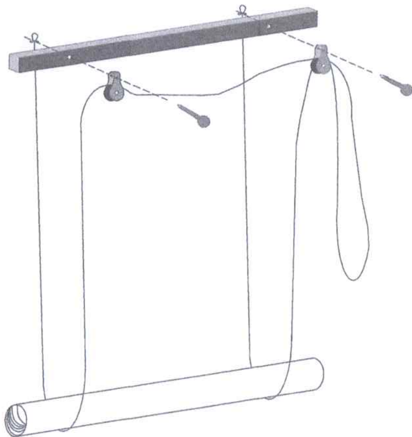
Roll Up Trapal with Pulley Details
